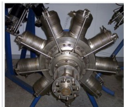
A 1917 Gnome 9N 160 hp Monosoupape rotary engine, with dual ignition provision. Diameter is 95cm (37.4 in)
